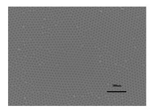
${\bf Fig.~3}-{\rm SEM}$  image of surface of AAO after 2nd anodization in sulfuric acid
