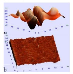
${\bf Fig.~1}-{\rm AFM}$  of Surface of the Al foil (a) before and (b) after the electropolish
