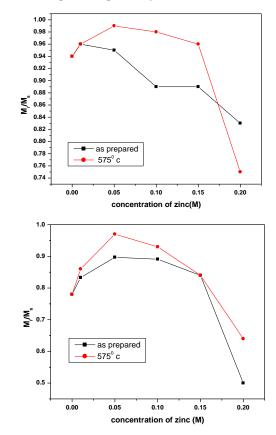
Fig. 7 – Squareness of nanowires with (a) 20 nm and (b) 35 nm diameter to concentration of zinc (M) before and after annealing in 575  $^{\circ}{\rm C}$
