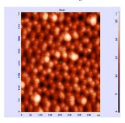
Fig. 2 – SEM AFM image of Surface of the AAO after remove the oxide layer in first anodization in sulfuric acid
