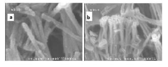
Fig. 4-a) SEM image of nanowires with 35 nm diameters and 2.1 mm length and (b) with 20 nm diameter and 2.5 mm length
