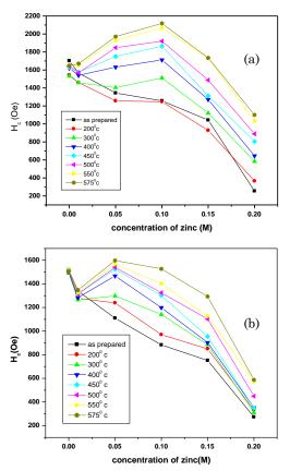
Fig. 6 – The coercivity of  $Co_{1.x}Zn_x$  nanowires with diameter of (a)20 nm and (b) 35 nm as a function of percentage of Zn and annealing temperature
