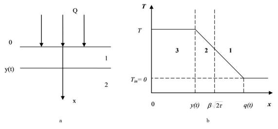
Fig. 1 – Heat flux incoming on metal surface (a) and temperature distribution in instant t (b)
