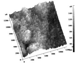
Fig. 2-3D photograph of relief in the peripheral lowintensity region at the titanium surface after irradiation by nanosecond ArF-laser with wavelength of 193 nm
