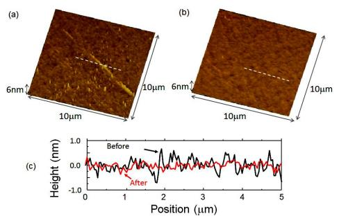
Fig. 2 – AFM images: (a) before and (b) after DPP etching. (c) Cross-sectional profiles along the dashed white lines in (a), and (b)
