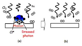
Fig. 1 – Schematic of DPP etching
