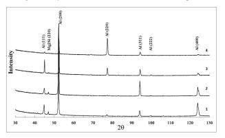
**Fig. 5** – X-ray diffraction patterns of the 6060 alloy in the initial state: after homogenization at 560°C for 12 h (1), after quenching from 480°C and aging at 185 °C for 6 h (2); after UIT: after quenching from 480°C and aging at 185 °C for 6 h (3), after homogenization at 560°C for 12 h (4).
