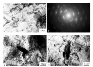
Fig. 3 – The inside of the homogenized 6060 alloy after UIT: the structure (a) and electron diffraction (b); interaction of the  $\beta$  phase particles with "flow" zones and the formation of loop-like configurations of ragged dislocation borders A (c) and cellular structure B (d).
