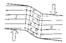
Fig. 1 – Scheme of the re-orientation band [11]
