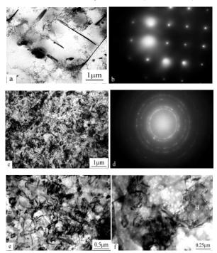
**Fig. 2** – The structure (a) and electron diffraction (b) of the homogenized 6060 alloy; the structure (c) and electron diffraction (d) of the surface after the UIT; the extinction dipoles A (e); the porosity and re-orientation bands with ragged edges B (f)
