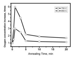
Fig. 1 – Time dependence of the relative oxygen concentration in the USJ region  $(10-50~\rm{nm})$  after furnace annealing
