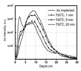
Fig. 2 – SIMS arsenic depth profiles before and after furnace annealing at 750  $^{\circ}\mathrm{C}$  for different times
