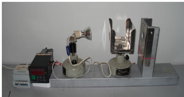
Fig. 3 – Optic and thermometric parts of measuring apparatus
