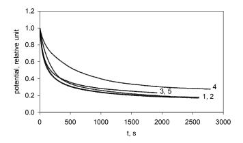
**Fig. 1** – The time dependence of the surface potential for the samples charged in the negative corona discharge.  $T = 70^{\circ}C$ . 1 – pure PE; 2 – PE + 2 vol.%; 3 – PE + 4 vol.%; 4 – PE + 8 vol.%; 5 – PE + 10 vol.% of talc
