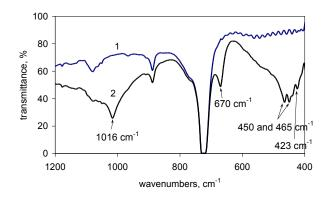
Fig. 2 – IR-spectra of pure polyethylene (1) and polyethylene with talc  $\left(2\right)$
