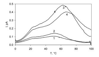
**Fig. 4** – The dependence of depolarization current from temperature for composite polymer. Temperature of polarization 70°C. 1 - pure PE; 2 - PE + 2 vol.%; 3 - PE + 4 vol.%; 4 - PE + 8 vol.%; 5 - PE + 10 vol.% of talc
