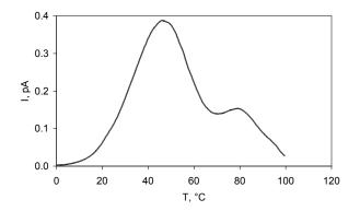
Fig. 3 – The dependence of depolarization current from temperature. Temperature of polarization 70°C.  $T_{max1} = 45^{\circ}C$ ,  $T_{max2} = 80^{\circ}C$
