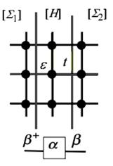
The model parameters  $\varepsilon$  and t are chosen in a way as to satisfy the standard dispersion relation with the effective mass. Finally
