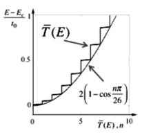
The approach we just described of viewing a 2D/3D conductor as a set of 1D conductors in parallel looks to us not only physically correct but also as a very powerful tool for interpretation of experimental data. Each of these 1D conductors is called a mode (or subband) and has a dispersion relation
