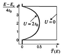
Another good example is that of a conductor with just one scatter whose effect is included in the Hamiltonian [H] by changing the diagonal element corresponding to that point to  $\varepsilon + U$ . Transmission through a single point scatter in a 1D wire with  $U = 2t_0$  is also shown above.
