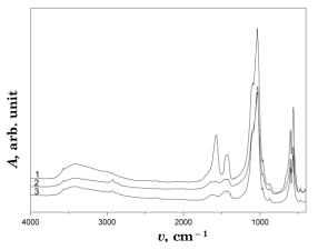
Fig. 1 – FTIR spectra of HAP (1), HAP-APS (2) and HAP-APS-AgNP (3)
