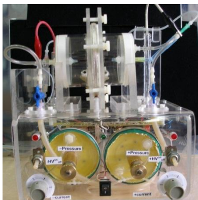
Fig. 2 – The latest prototype of a generator for production of biological nanoaerosol. Air pumps and flow meters are not shown in the picture
