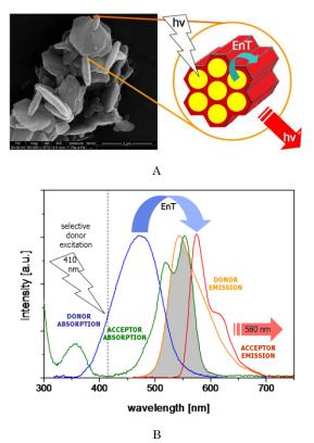
**Fig. 1** – A) SEM image and schematic representation of SBA-15 silica platelets loaded with SY polymer and functionalised with IRIS3 dye; B) absorption and emission spectra of both donor and acceptor chromophores: the overlap area is high-
