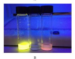
**Fig. 2** – A) photoluminescence emission spectra of the IRIS3-SY@SBA-15 system (red line) compared with SY@SBA-15 (yellow line) and IRIS3@SBA-15 (black line), all recorded from 0.5 mg/ml 2-propanol suspensions upon excitation at 410 nm; B) digital photographs under UV light of, from left to right, SY@SBA-15, IRIS3@SBA-15 and IRIS3-SY@SBA-15 in 2propanol suspensions
