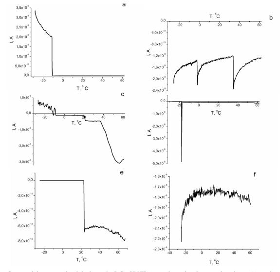
Fig. 2 – Spectra of thermostimulated discharge for  $InSe<CS(NH_2)_2>$ , synthesized under normal conditions (a), in the magnetic field (b), under the light (c) and in the electric field (d). (e) and (f) is  $InSe<CS(NH_2)_2>$  synthesized in a magnetic field and after 5 and 15 min. of ultra-sound irradiation, respectively
