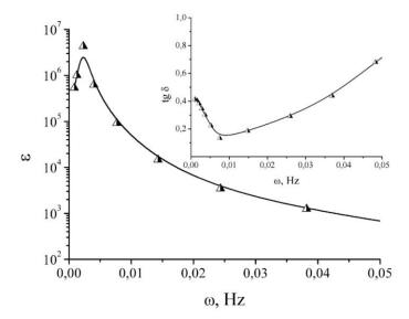
Fig. 3 – Infra-low-frequency dependence of the dielectric constant and the dielectric loss tangent (inset) for  $GaSe<CS(NH_2)_2>$ , synthesized under illumination. Measurements is in the magnetic field
