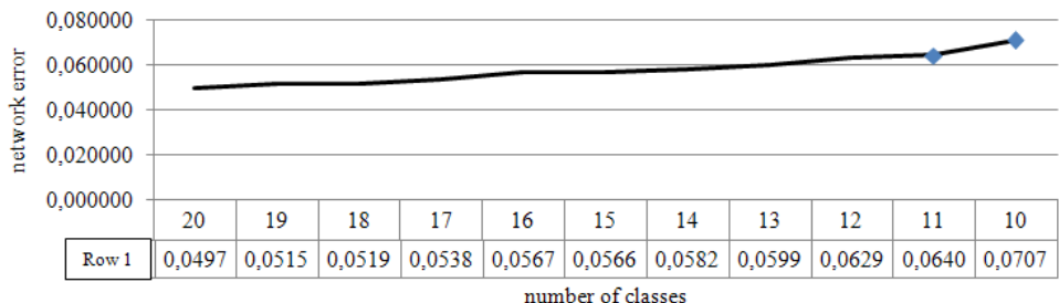
Fig. 4. Dependence of the Kohonen network error change on the number of identified classes (from 20 to 10)
