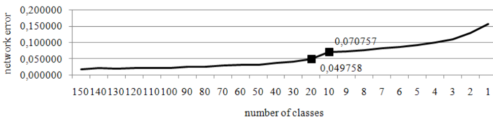
Fig. 3. Dependence of the Kohonen network error change on the number of identified classes (from 150 to 1)
