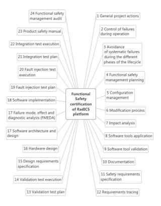
Fig. 7. General Assurance Case diagram for AC DD of FPGA-based safety platform RadICS
