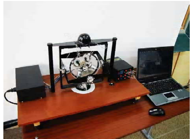
Fig. 10. Exterior view of HSC for research models and methods of maintenance the active fault-tolerance spacecraft attitude control and stabilization
