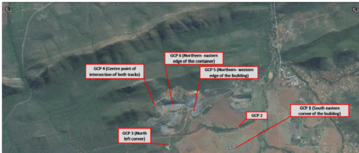
Figure 3. Six GCP points recorded for correct Georeferencing of the digital data
