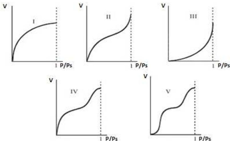
$V$  – adsorbed gas content,  $m^3/t$ ;  $P/P_s$  – ratio of pressure to vapor saturation pressure
