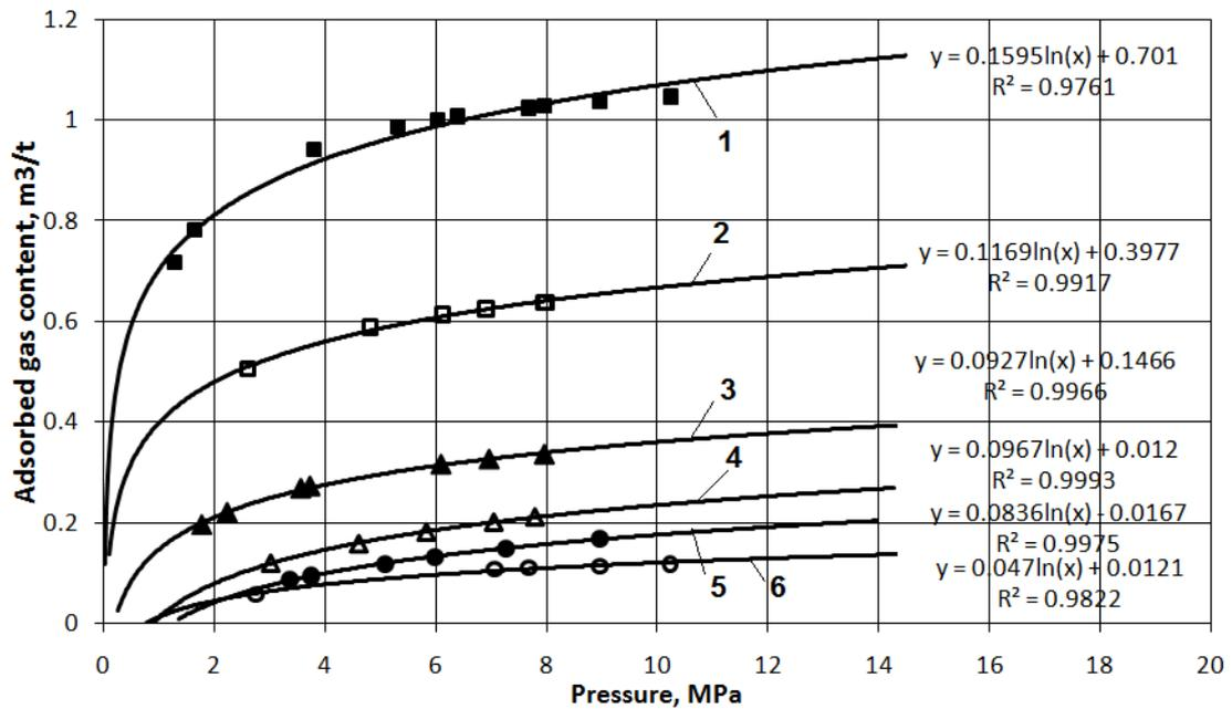
1, 2 – adsorption isotherms for the model with permeability of 9,7mD at temperature 40 °C and 60 °C respectively;
