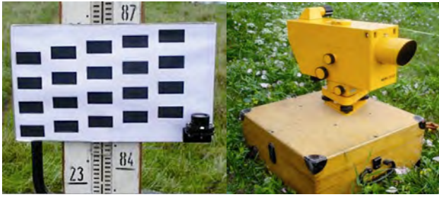
Fig. 7. Leveling mark and optical leveler Ni 002
