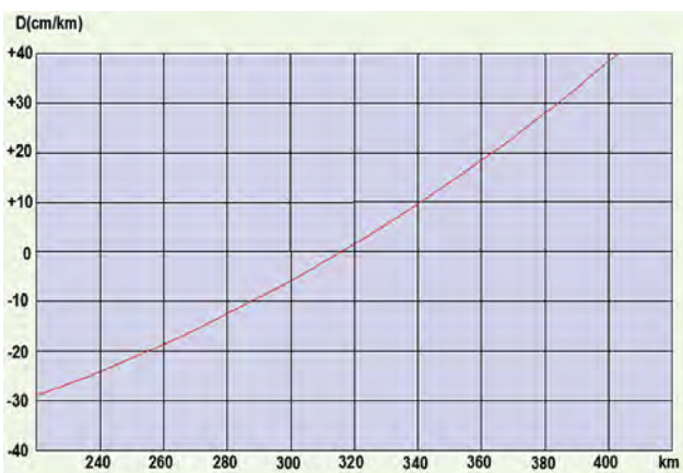
Fig. 6. Diagram of relative linear deformations for Stereo 70 map projection
