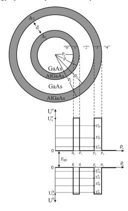
Figure 1. Cross-section and energy scheme of multi-shell nanotube.
