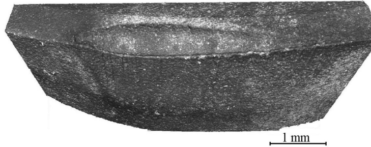
Fig. 6. 3D view of worn BCBN tool.
