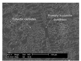
Fig. 1. Typical microstructure of HCCI material in lower C-Si group and as-cast condition.
