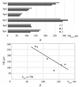
Fig. 5. Influence of materials on tool wear (a) and the correlation of  $h_{\text{max}}$  with tool wear in machining (b):  $v_c = 120$  (1), 140 (2), 160 (3) m/min.
