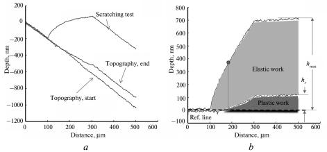
Fig. 2. The calibrated scratch test of fused silica sample by the load of 100 mN, test curve with topography effect (a), the analytical curve by removing of topography effect (b).
