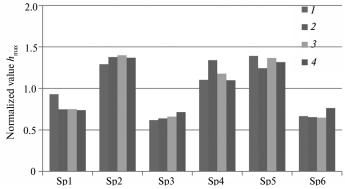
Fig. 4. Relative value of  $h_{\text{max}}$  represent wear performance features of HCCI materials by the load of 10 (1), 100 (2), 200 (3), 300 (4) mN.
