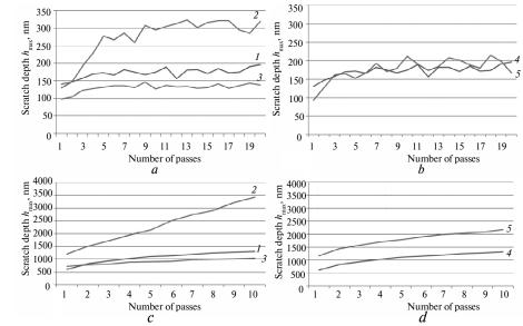
Fig. 3. The results of the sequential multi-passes tests on pre-worn surfaces: heat treatment effect by 10 mN (*a*), composition effect by 10 mN (*b*), heat treatment effect by 100 mN (*c*), composition effect by 100 mN (*d*): as cast (*1*), annealed (*2*), hardened (*3*), lower C–Si (*4*), higher C–Si (*5*).
