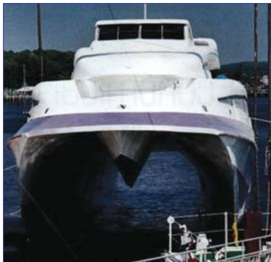
Fig. 4. Planning Catamaran with Interhull Bridge of Wedge-shaped Form and Internal Rounding Frames
