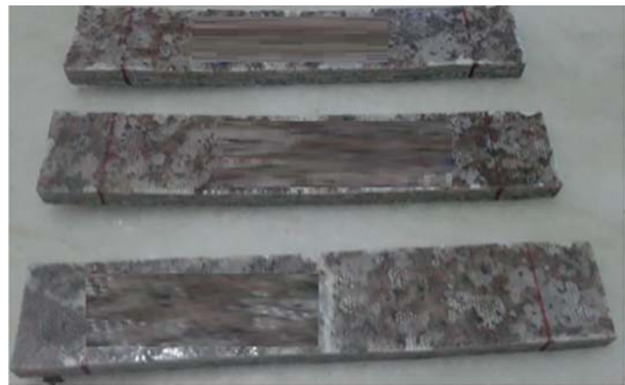
Specimens made from epoxy and basalt fibers
