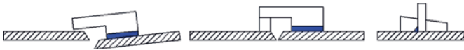
Figure 7. Weld clip along one edge only so it may be removed easily with a hammer. Drive steel wedge below clip until plate edges are in alignment
