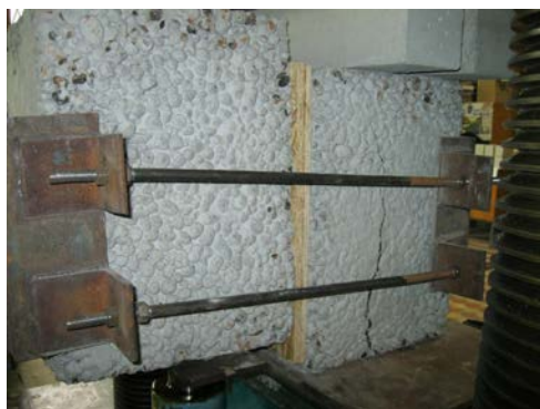
Pic.5. The formation of the cracks in the concrete prisms
