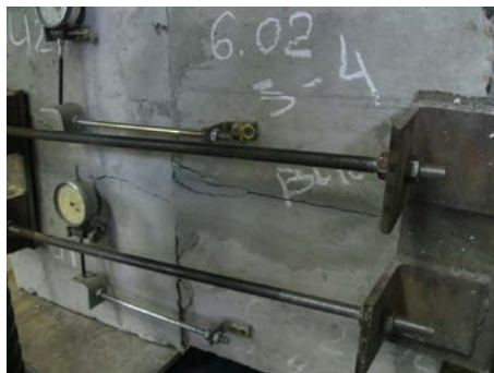
Pic.4. The formation of the cracks along the contact of the mortar joint
