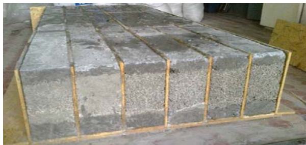
Fig. 1. Test specimens of three-layer beams
