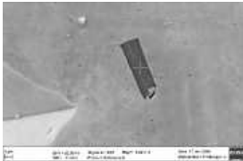
Fig.9 Another Ti(C,N) particle before heating
