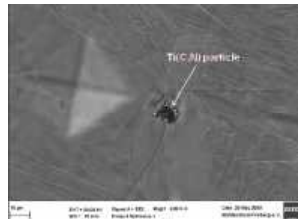
Fig. 7. The same Ti(C,N) particle after heating and cooling
