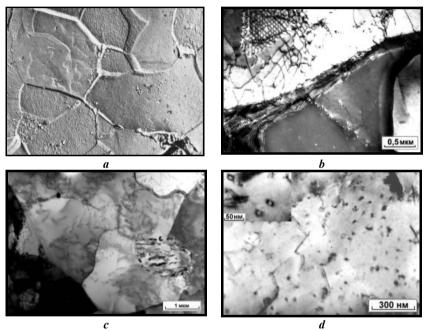
**Figure 4.** Thin structure in 22 mm thick plates of low-carbon steel 10G2FB rolled by the experimental schedule: a, b, c – electron microscope image of subgrain (polygonal) boundaries; d – dispersed carbides of (Nb, V)C type in ferrite
