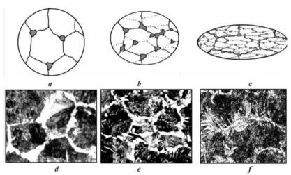
**Figure 2.** Sequential stages of  $\alpha$ -crystal nucleation at polygon boundaries at temperatures reduced down to the values below point  $Ac_3$ ; d-f: precipitation of hypoeutectoid ferrite in steels which underwent austenite decomposition after cooling in air, ×800: d: from a single heating by 1050 °C, e: after 16% hot reduction at 1000 °C; f: after 36% hot reduction at 1000 °C.
