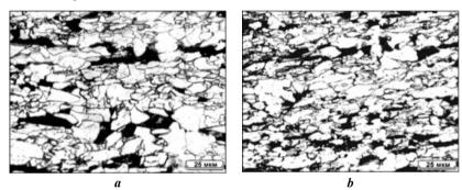
**Figure 3.** Structure of 22 mm thick plates of low-carbon steel 10G2FB rolled by conventional technology (a) and with the use of the proposed schedule (b)
