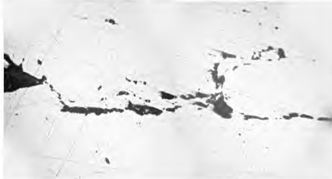
Fig.1. Sulphide inclusion fracture, \times 150 .
