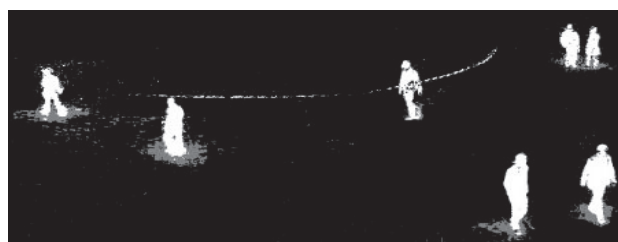
Fig. 2. Foreground mask obtained using MOG2 Background Subtractor
