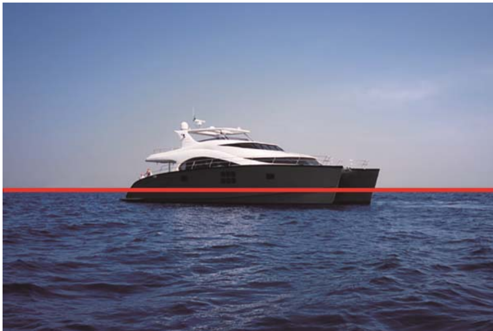
Fig. 6. The detected sea-sky-line
