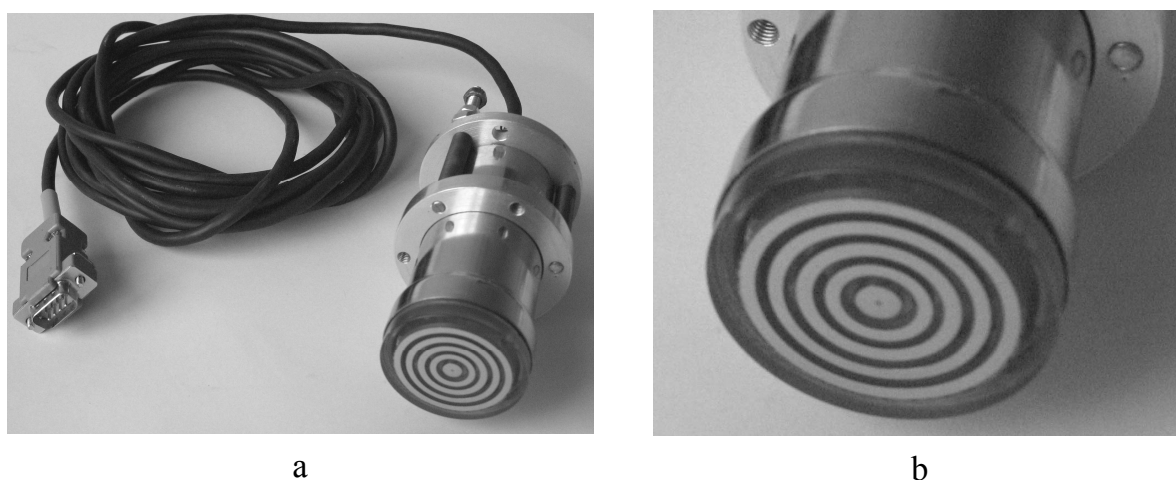
Figure 1 – PMT with integrated to him the contact capacitive sensor: a – general view of PMT; b – sensor (increased)
