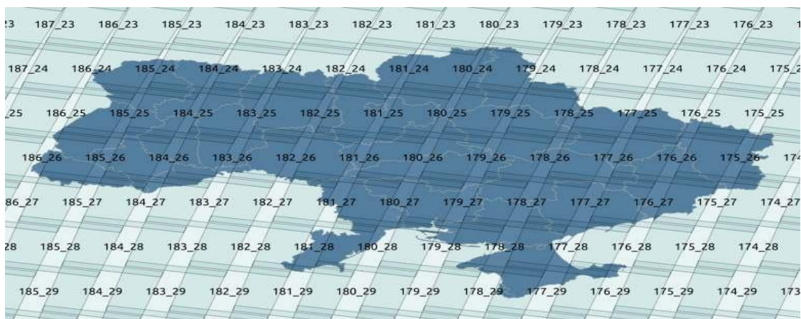
Figure 2 - Visualization of the coverage of the territory of Ukraine with Landsat 8 imagery following WRS-2
