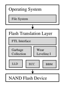
Fig. 3. Software for an embedded system using a NAND Flash memory
