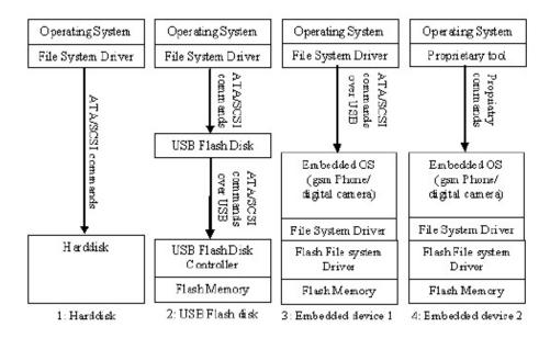
Fig. 2. Components involved in hard disk and flash memory access
