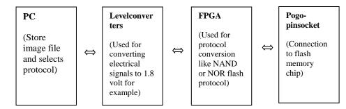
Fig. 4. Schematic of NFI memory toolkit
