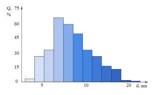
Figure 6 – Distribution of quantum wires by dimensions: Q is the share of particles, %; d – dimensions of particles, nm
