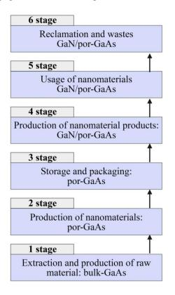
Figure 4 – Life cycle of porous gallium arsenide and gallium nitride based on it
