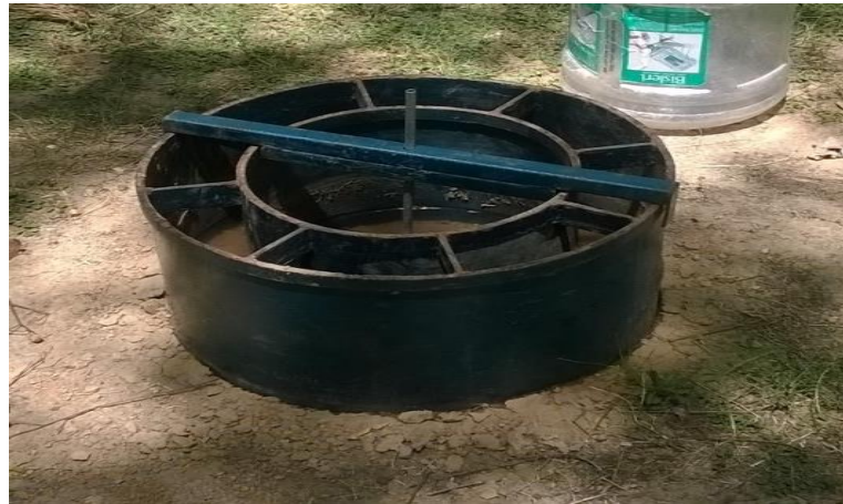
Figure 2 – The Double ring infiltrometer having 300 mm inner diameter and 450 mm outer diameter for measuring infiltration rate
