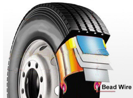
Fig. 1. The bead wire and its placement
