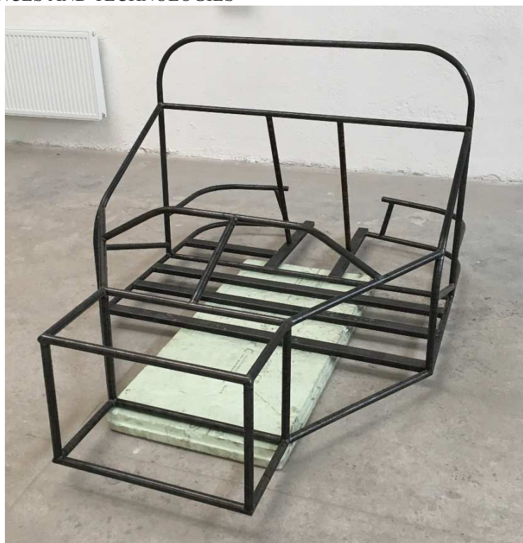
Fig. 3. Frame of pneumobil
