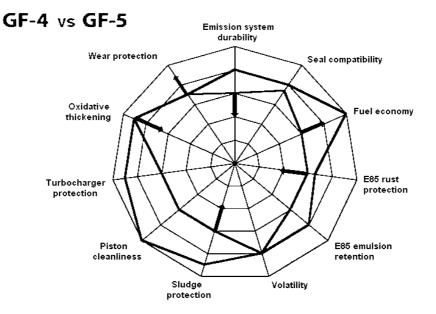
*Figure 2*. Changes in the performance spectrum of ILSAC GF-4 oil top-treated with IF-WS2 emulsion
