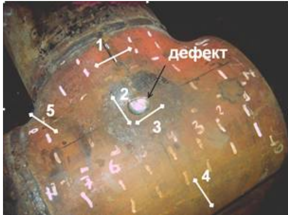
Figure 1. General view of the T-joint with outer artificial defect (the arrows indicate the cutting directions of the specimens in zones 1, 2 – 3, 4 and 5)
