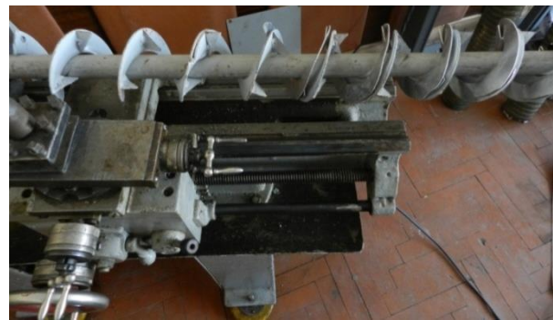
Figure 3. WSCP manufacturing with screw mandrel
