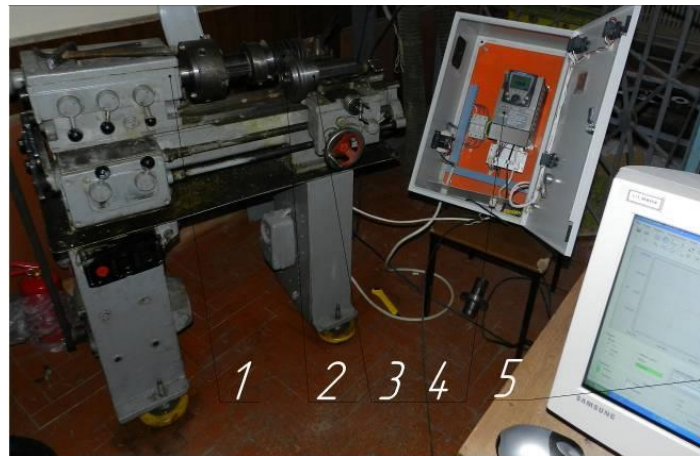
Figure 8. General view of stand equipment: 1 – machine; 2 – SB; 3 – shaping tool; 4 – Altivar; 5 – PC
