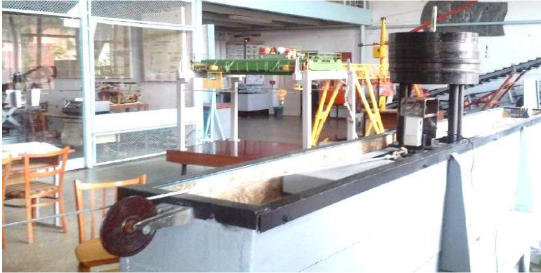
Figure 7. The experimental stand for the interaction research of the skis supporting surface and the stepping motor with the ground
