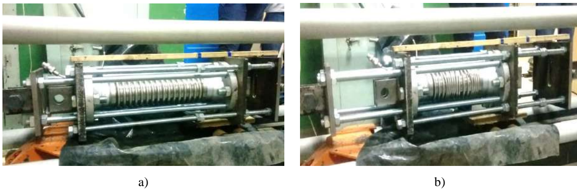
Figure 5. The compensator during testing
