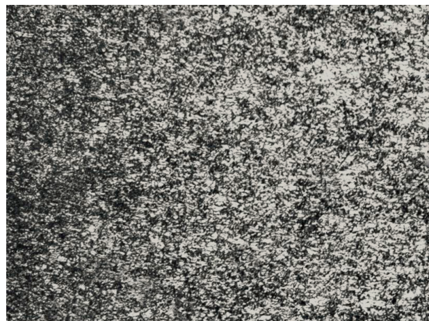
Fig. 5. Microstructure of recrystallization area of a heat affected zone in the weld joint ( \times 300 )
