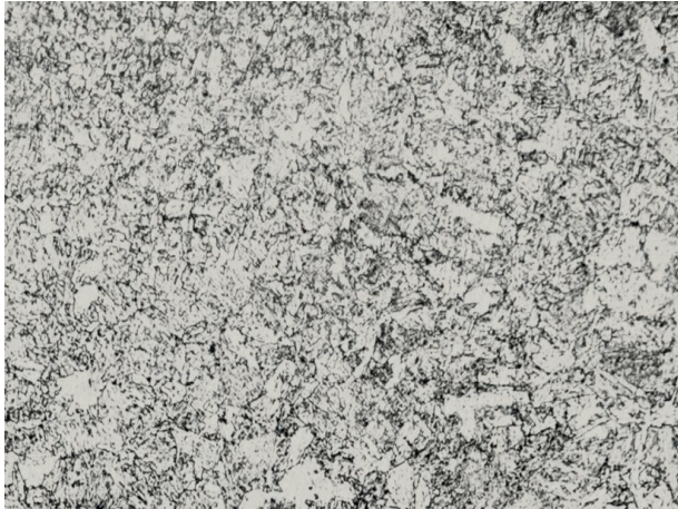
Fig. 6. Microstructure of the total recrystallization area of a heat affected zone in the weld joint (x 300)
