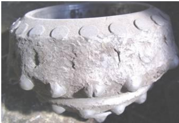
Fig. 1. Appearance of the destroyed roller three-cone drill bit
