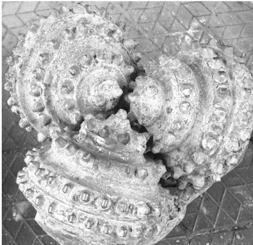
Fig. 1. Appearance of the destroyed roller three-cone drill bit
