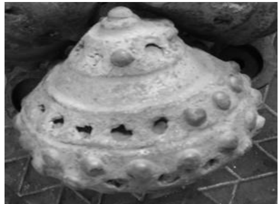
Fig. 1. Appearance of the destroyed roller three-cone drill bit
