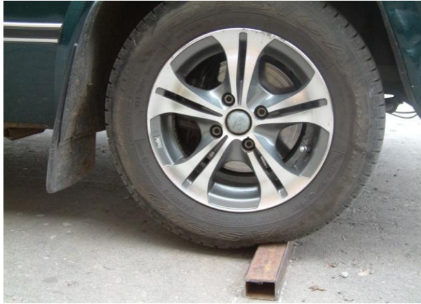
Fig. 3. Photo of the car's tire hits the one-time obstacle
