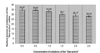
**Fig. 2.** Surface tension of solutions of the "San-active" depending on its concentration
