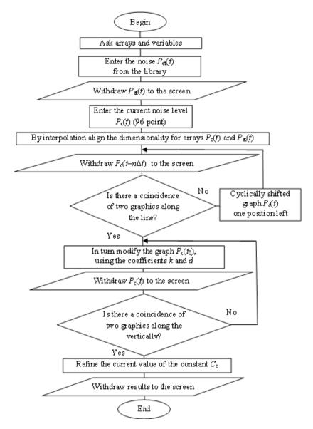
Fig. 1 – The flowchart of algorithm for correction of constant  $C_{\rm c}$
