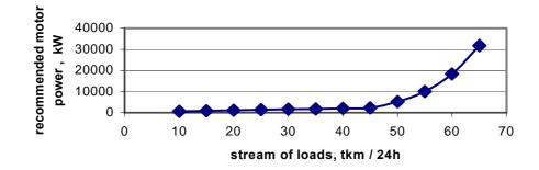
Fig. 5. Optimal motor power depending on evaluate difference of streams of loads
